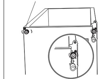
9. Unscrew and remove the bottom hinge pin, turn the bracket over and replace it.
